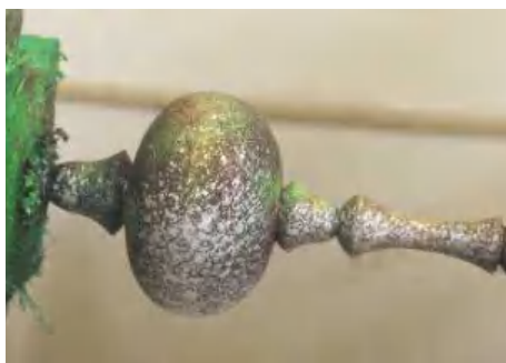
▲ Pic.10 Next, spray some gold and silver paint onto the work and you will find this gives you an interesting mottled effect, which I think looks really good
